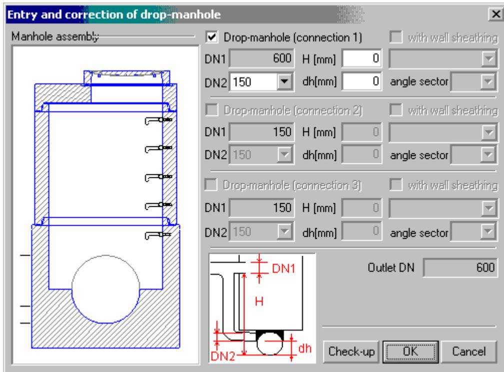
Fig. 16 – dialog for entry and correction of a drop-manhole data
