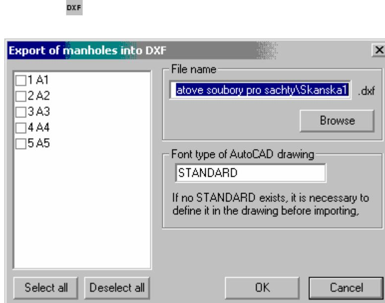
Fig. 4 – dialog for export of manholes into DXF
