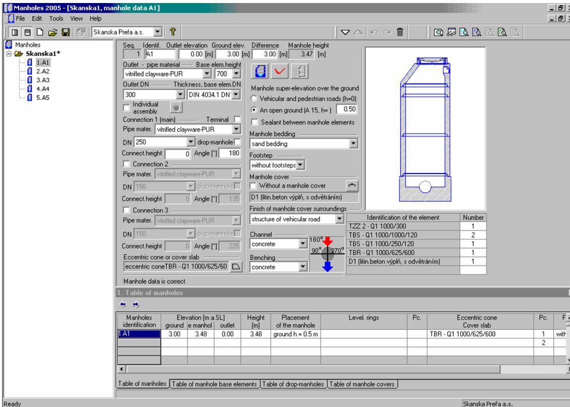
Fig. 1 – user's interface of the “Precast Sewer Manholes 2005” program
