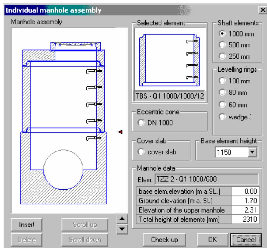
Fig. 15 – dialog for individual assembly of a manhole
